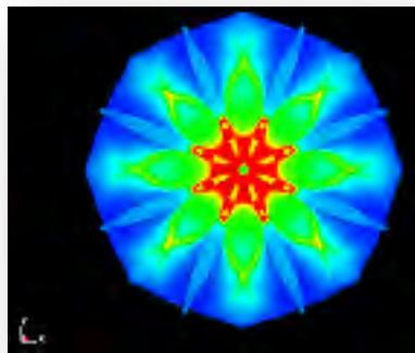
Plane detonation wave collision analysis using ALE method
